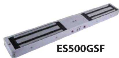
500kg/1200lbs, Surface mounted, double door LED, feedback(NO/NC/COM), timer
